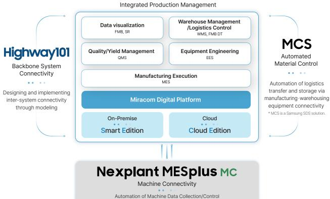
\* FMB : Flexible Monitoring Board | SR : Smart Report | WMS : Warehouse Management System | FMB DT : Flexible Monitoring - Board Digital Twin QMS : Quality Management System | EES : Equipment Engineering System | MES : Manufacturing Execution System MES : Manufacturing Execution System | MCS : Material Control System | MC : Machine Control
